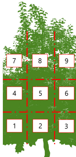
Fig. 1. Placement of water-sensitive papers in different canopy sections for spray coverage analysis. Water-sensitive papers were attached to different canopy sections of the tree to assess spray coverage. The canopy was divided into nine distinct zones: lower (0.0-1.5 m), middle (1.6-3.0 m), and upper (3.1-4.3 m) parts of the tree.
